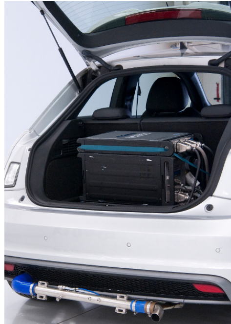
>> PEMS equipment setup in trunk of Audi A1
